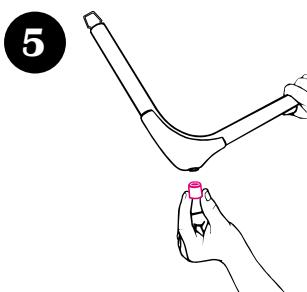
Tap leg tips on the floor to be sure they are completely on.
